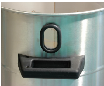
Sight Glass on Recovery Tank
